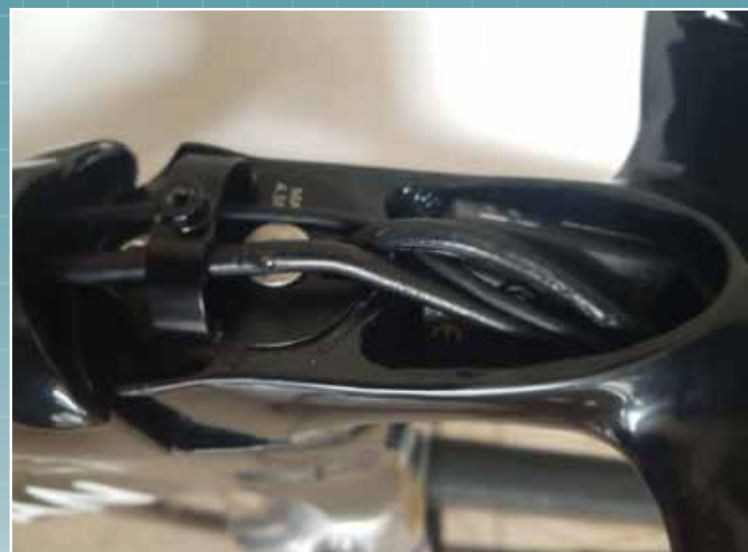
The Di2 buried controller and internal ducts passages
